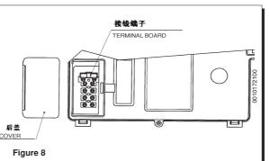
A 2A fast-blowing fuse is incorporated in the power supply terminal block (to check or replace the fuse, pull out the black fuse carrier).
