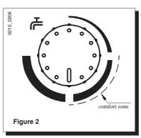
The gas valve is provided with an electronic flamemodulating function, which operates depending on the DHW temperature adjusting control (6) settings and on the quantity of water drawn from the taps. This electronic device allows to keep the water coming out of the boiler at a constant temperature
