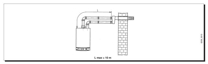
A 90° bend reduces the total duct length by 0.5 metre.
