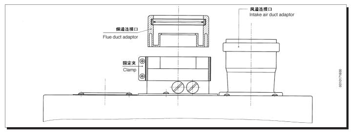
在管道能够旋转 360°的情况下,90°弯头可以在任何 方向连接在壁挂炉与烟气一空气管道上。并且,它可 以用作一个备件,连接管子或一个 45°弯头。 The 90° bend allows to connect the boiler to flue-air ducting regardless of direction as it can be rotated by  $360^\circ$ . It can moreover be used as a supplementary bend to be coupled with the duct or with a  $45^\circ$  bend.
