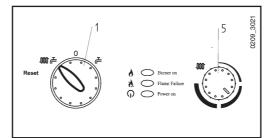
**Warning**: When the selector switch (1) is set on Wintertime operation ( $\bigcap \cap \vdash$ ) it may be necessary to wait some minutes at each intervention of the central heating temperature adjusting control (5). To relight the main burner immediately place the selector switch (1) on (0) and then again on ( $\bigcap \vdash \vdash$ ). No waiting is needed when the boiler is in the DHW mode on models with this option.
